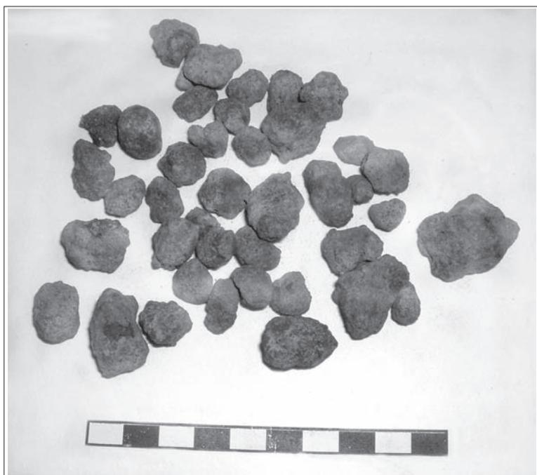
Fig. 2. Hydrated iron ore from Lieporiai.
